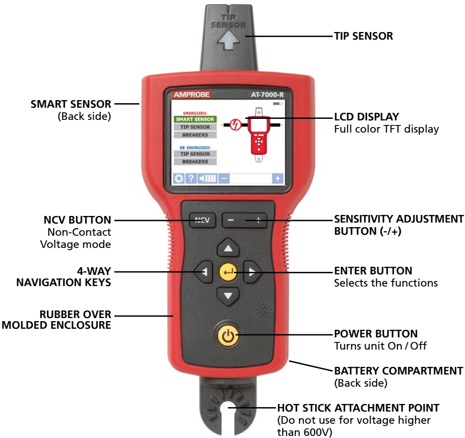
Figure 1: Overview of AT-7000-R Receiver
