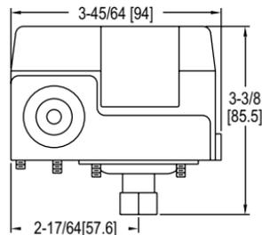
The **Series CXA Water Pump Pressure Switch** has been proven reliable for controlling automatic water systems. These switches are very popular for use on water well pumps and pumping systems. The set point and dead-band are both easily adjustable via screws inside the cover. For ease of installation, the switches come with a 1/4" female NPT process connection and can be mounted in any orientation. The series CXA's simple design makes it a great switch for an installer at any skill level.
