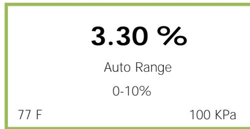
The display will shift to the next higher range when the oxygen reading (actually the sensor's signal output) exceeds 99.9% of the upper limit of the current range. The display will shift to the next lower range when the oxygen reading drops to 85% of the upper limit of the next lower range.
