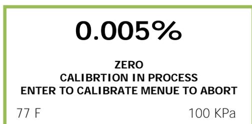
Pressing ENTER, the analyzer will complete ZERO calibration and return to Sample mode. If you press ENTER when the oxygen reading is outside of the acceptable zero offset limit, the analyzer will fail ZERO calibration and return to the Sample mode.
