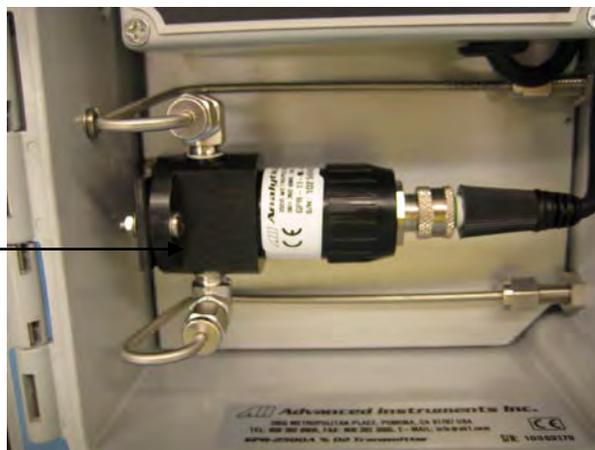
Flow rates of 1-5 SCFH cause no appreciable change in the oxygen reading. However, flow rates above 5 SCFH generate backpressure and erroneous oxygen readings because the diameter of the integral tubing cannot evacuate the sample gas at the higher flow rate. The direction the sample gas flows is not important, thus either of the two tube fitting connectors can serve as the inlet or vent.
