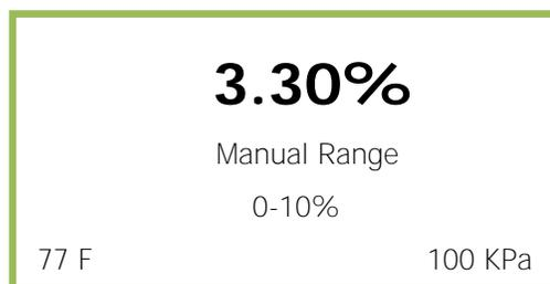
The display will not shift automatically. Instead, when the oxygen reading (actually the sensor's signal output) exceeds 110% of the upper limit of the current range an OVER RANGE warning will be displayed.
