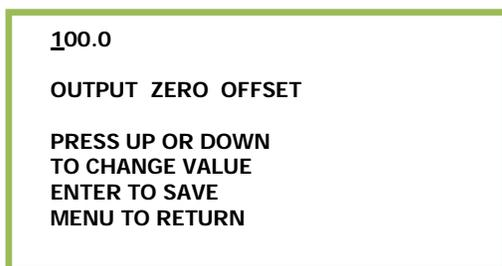
The default setting of 100 illustrates no adjustment to the analog output signal. Compute the adjustment value as described in Appendix B or consult the factory. The true adjustment value must be determined empirically by trial and error. Adjust the initial value to above 100 to increase the analog signal value or decrease it below 100 to decrease the analog signal.
