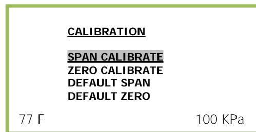
Press the ENTER key to select the SPAN CALIBRATE option. The following display will appear.
