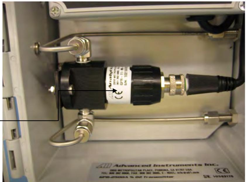
Delrin Housing with Oxygen Sensor installed
