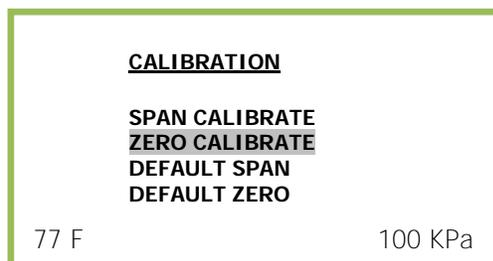
Allow the zero gas to flow through the transmitter until a stable oxygen reading is obtained. This may take from several minutes to a few hours. It is highly recommended to monitor oxygen trend on a chart recorder to ensure that the oxygen reading has stabilized; evidenced by a horizontal trend.
