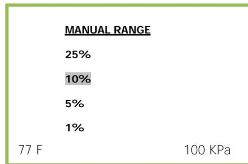
Advance the reverse shade cursor using the ARROW keys to highlight the desired RANGE.
