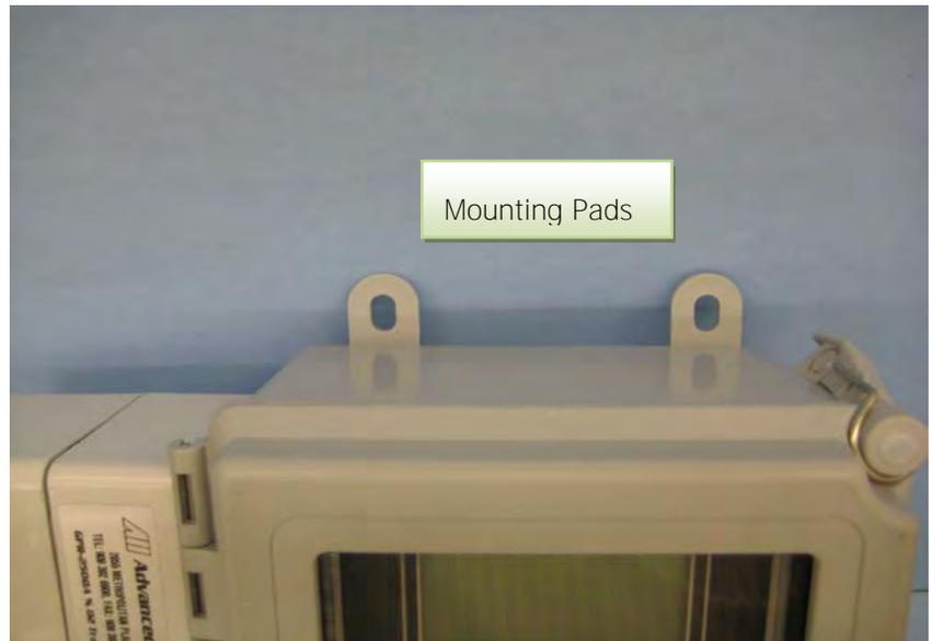
The GPR-2500A is housed in a Fiber Glass NEMA4X rated enclosure. This configuration is designed to be mounted directly to any flat vertical surface, wall or bulkhead plate with four (4) of the appropriate size screws. To facilitate servicing the interior of the transmitters, position it approximately 5 feet off ground level.
