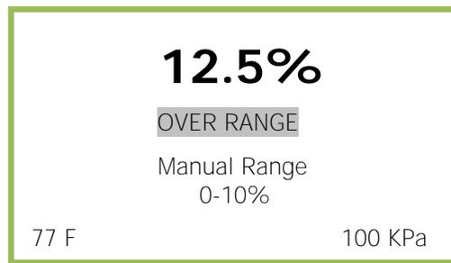
Once the OVER RANGE warning appears the user must advance the transmitter to the next higher range via the menu and keypad Press MENU, select MANUAL SAMPLING, press ENTER, select the appropriate MANUAL RANGE and press ENTER again.
