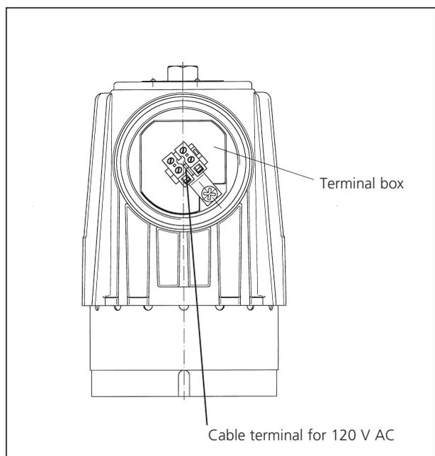
• Dimensions and components of Lumiglas luminaires USL 08-Ex:
