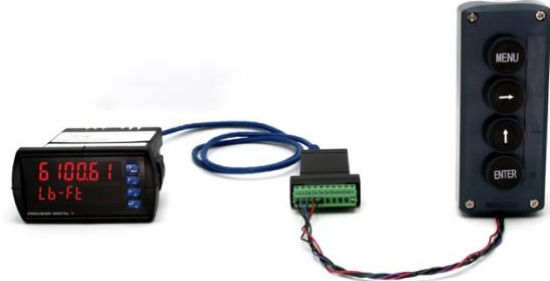
Figure 29. Meter to Control Station Connection
