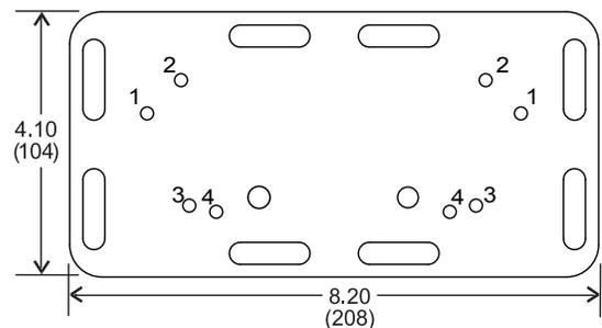
Figure 2. Hole Location Table & Dimension Drawing: Inches (mm)
