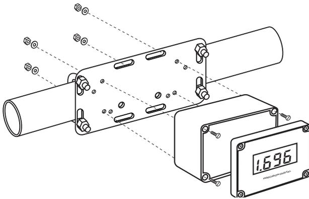
Figure 4. PDA6845 with PD686 Mounted to 2" Horizontal Pipe
