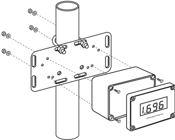
Figure 3. PDA6845 with PD686 Mounted to 2" Vertical Pipe
