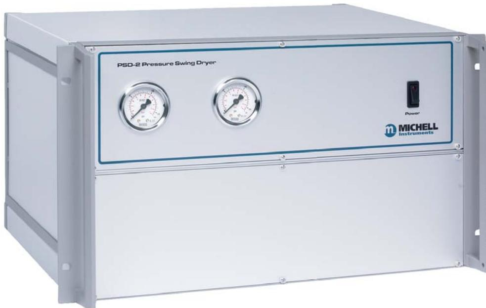
The Michell PSD Series Pressure Swing Dryers use two columns filled with 4Å molecular sieve desiccant, which are used alternately on a switching cycle. The PSD dryers are designed to operate continuously, using a small proportion of the dried air to regenerate the offline column - generally giving desiccant life in excess of five years. This type of heatless regeneration uses significantly less energy than a 'heated' dryer.
