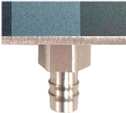
Figure 3.2 Connections on bottom right of instrument (vacuum connection)
