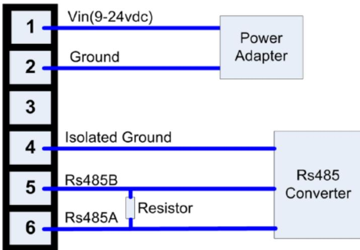
Figure 3.5 Application for a single sensor
