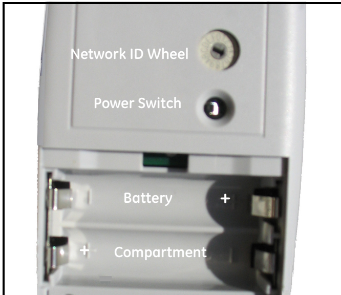
Figure 4: Logger Battery Compartment, Power Switch and Network ID Wheel
