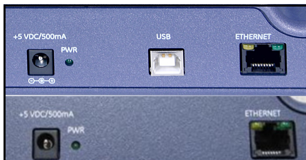
Figure 5: Base Station Connections (old and new)
