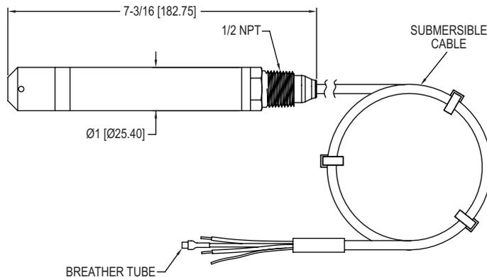
The Series SBLT2 & SBLTX Submersible Level Transmitters are manufactured for years of trouble free service. These series measure the height of liquid above the position in the tank referenced to atmospheric pressure. The transmitter consists of a piezoresistive sensing element, encased in a 316 SS housing.
