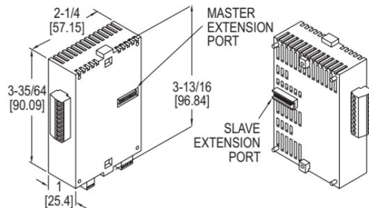
The **Series SCD DIN Rail Temperature/Process Controllers** offer multiple PID loops in a compact size. Each SCD-1000 master controller can be combined with up to seven SCD-2000 slave controllers without any wires. Each controller has one universal input, one relay output and one user selected output.
