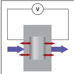
The MSRS responds quickly to oxygen and has a T90 of under 11 seconds. Another benefit of having a sealed reference is that measurements can be made without a reference gas and independent of the quality of the surrounding air. The analyzer is virtually drift-free, extending calibration interval time.
