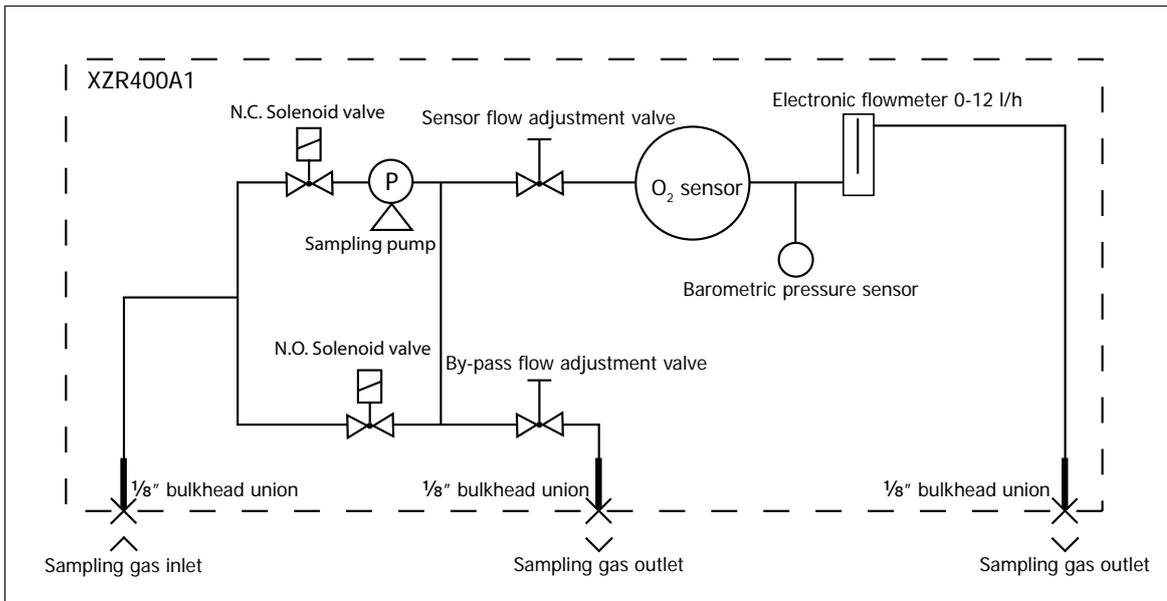
Figure 17 *Sample Path with Pump Fitted XZR400A1*
