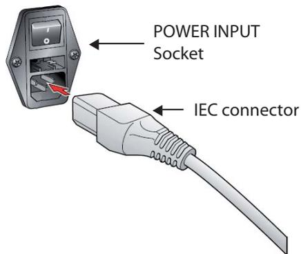
Figure 28 *Power Input Socket*
