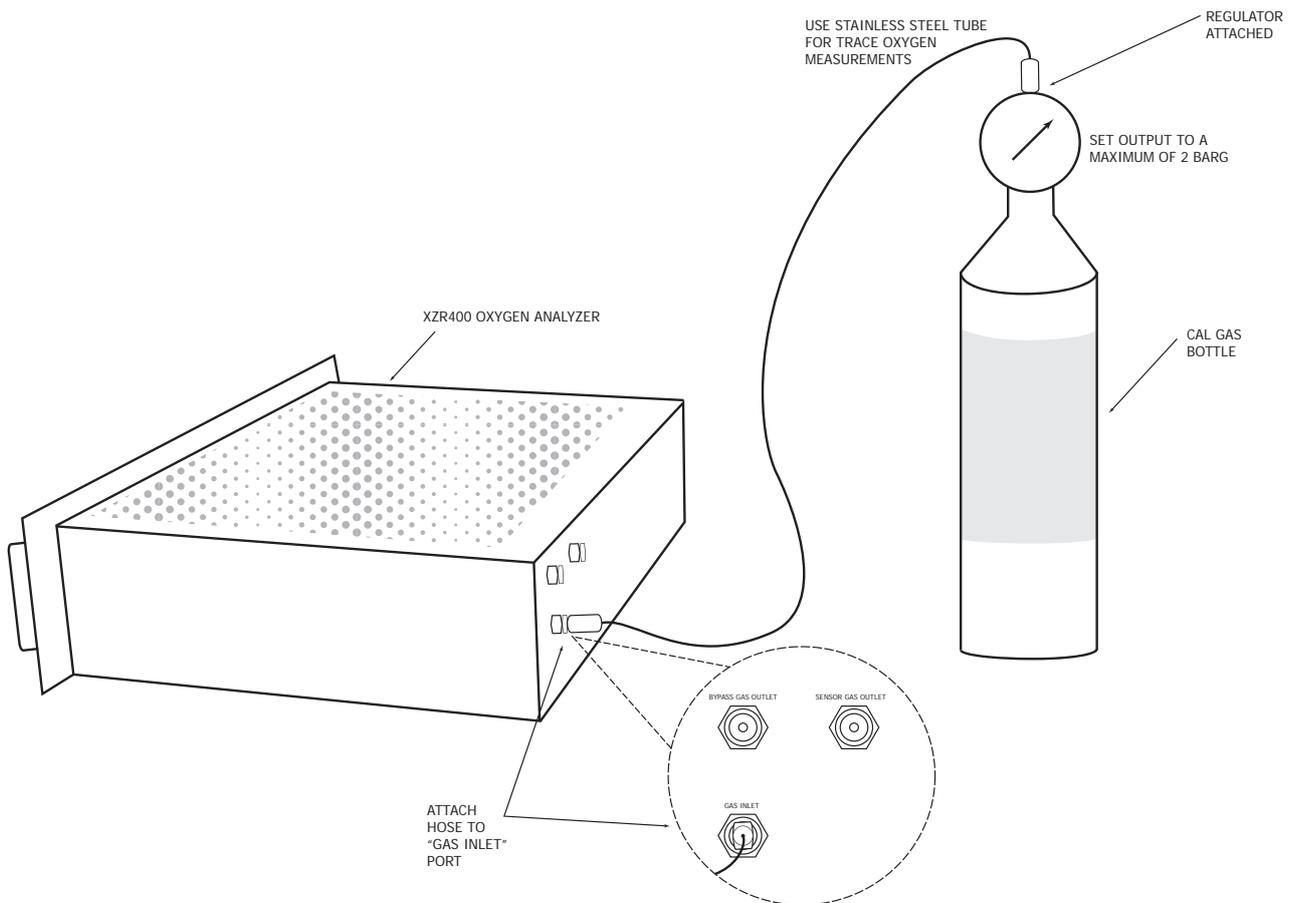
Figure 44 Calibration Procedure with XZR400A1
