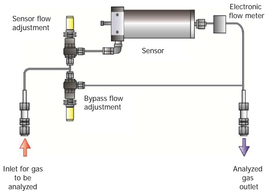
Figure 19 Gas Circuit Diagram for XZR400A2
