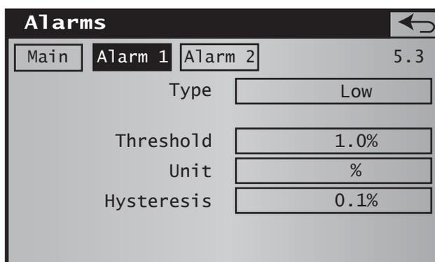
Figure 39 Alarm Screen (Alarm 1)
