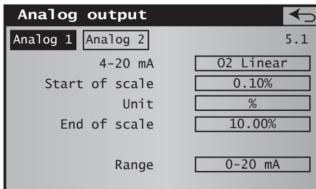
Figure 37 Analog Output Screen
