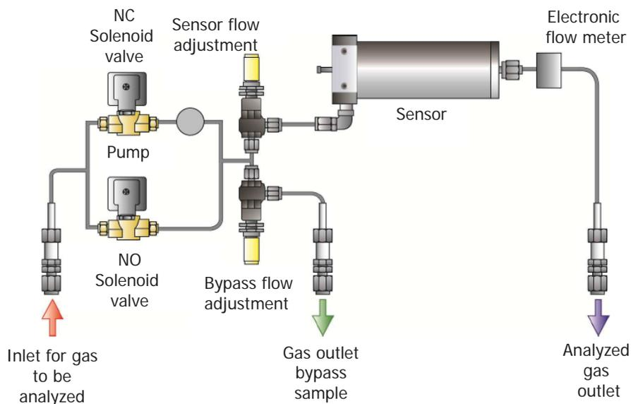
Figure 14 Gas Circuit Diagram for Rack & Pump Version
