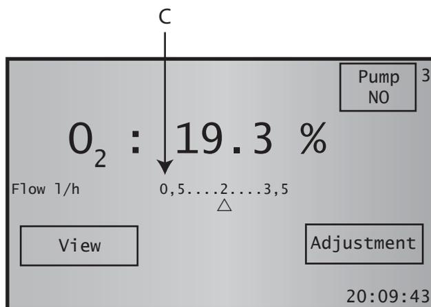
Figure 31 Sample Flow Adjustment
