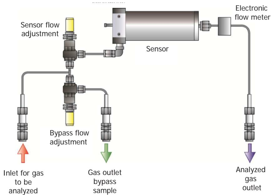
Figure 13 Gas Circuit Diagram for Rack Version
