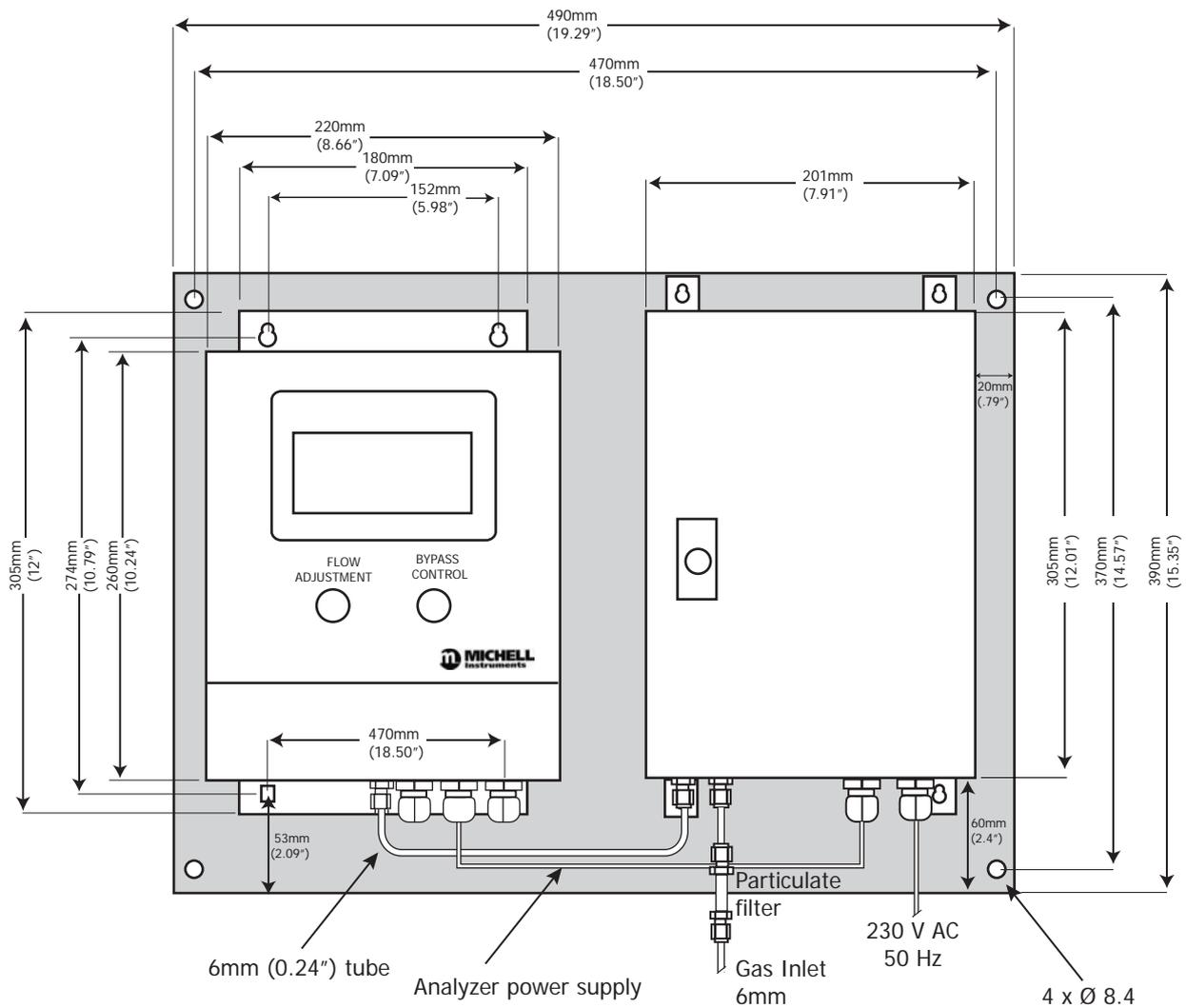
Figure 8 Dimensions - ZXR400A2 with External Pump Option
